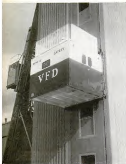
A NEW ESCAPE SYSTEM is called Sky Van. The elevator car clips onto exterior vertical rails, is self-powered. It can carry 4500 pounds up or down
